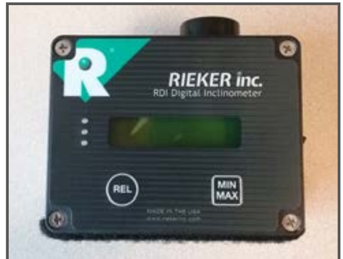
Traditional and digital ball bank indicators (Photos: Courtesy of Kansas LTAP and Iowa LTAP)
