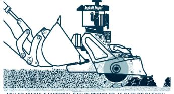
MILLED 1" MINUS MATERIAL CAN BE RECYCLED AS BASE OR BACKFILL
