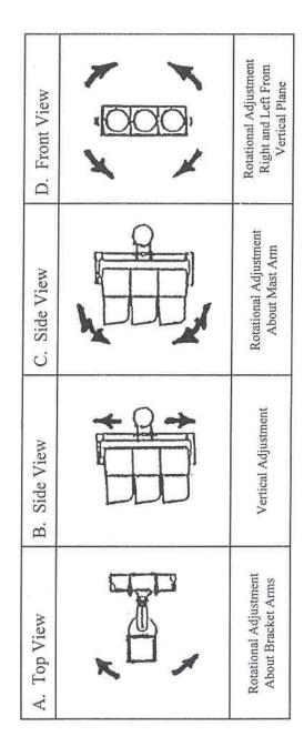
Figure 921-1: Signal Head Bracket Adjustment
