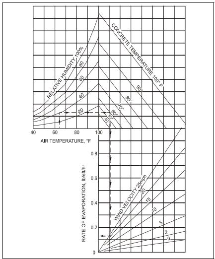
Figure 706-1: Surface Evaporation for Concrete
