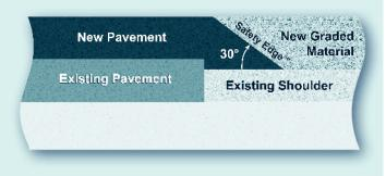
With the *Safety Edge*, as the shoulder material settles or erodes, a 30 degree taper provides a gradual and safer transition between pavement and shoulder for autos, motorcycles, and bicycles.
