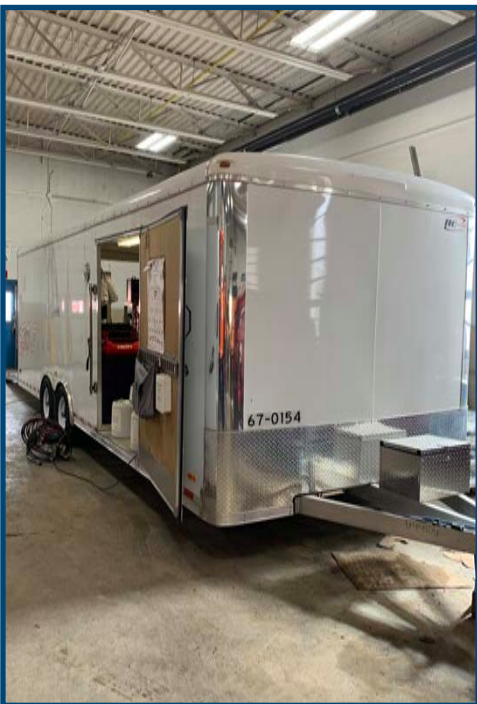
Outside view of the epoxy injection rig, built in 24-foot trailer (Photo: Courtesy of MDOT)
