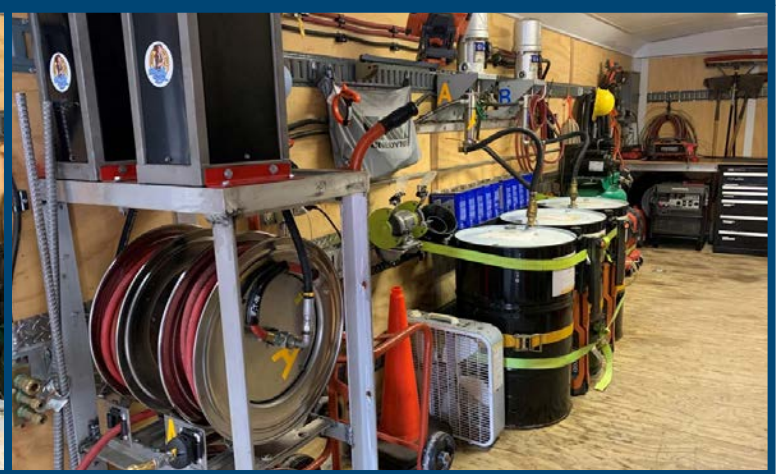
Inside views of the epoxy injection rig built by Porter and Graves and used to transport tools and material for epoxy crack and deck injection and polyurethane sealing. Top Left: Back end of trailer with injection pumps on left. Top right: Front end of trailer with workbench. Bottom Left: Transfer pumps. Bottom Right: Views of injection pumps, transfer pumps and drums, and workbench. (Photos: Courtesy of MDOT)
