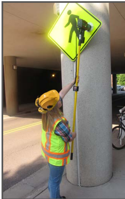
Testing the retroreflectivity of a sign using a reflectometer (Photo: CTT Archive)
