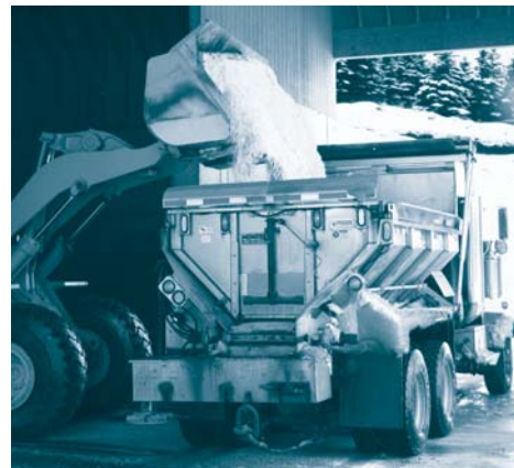
A Manistee County Road Commission (MCRC) truck stops for a new load of salt. MCRC uses a combination of materials for pre-wetting their salt. “No single product or material will solve every problem,” Jerry Peterson, manager of MCRC, said.
