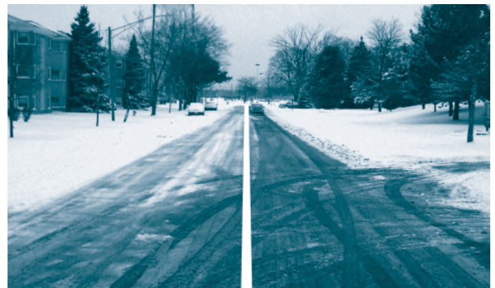
Anti-icing involves applying a salt brine or similar material to a roadway before a snow event to keep ice and snow from bonding to the pavement. The right lane of the road above was treated with 85% brine, 10% Geomelt and 5% Calcium Chloride. The left lane was not treated.
